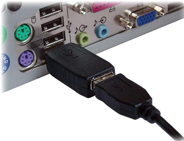
Connect the hardware USB keylogger between the USB keyboard and the USB port. Keystroke logging will start automatically.
